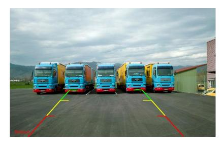
When the astern signal line is triggered, the camera view of channel 4 is automatically displayed along with the astern line.
